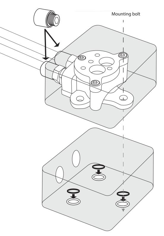
The built-in-box is placed on the floor, so the top is alligned with the surface of the floor.
