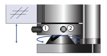
The 2 pinol screws are used to set the zero point of the raising/lowering feature
