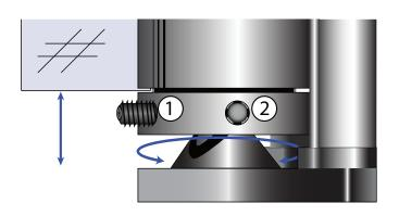
The 2 pinol screws are used to set the zero point of the raising/lowering feature
